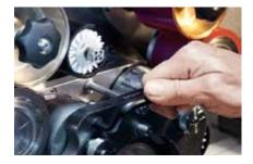
**Never unstuck:** the sensor monitors the tipping paper to ensure that it is always correctly glued.
